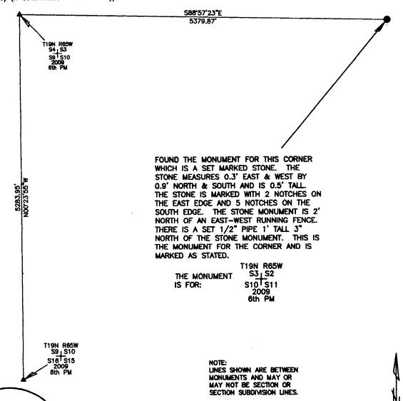
THE MONUMENT FOR THIS CORNER IS A SET MARKED STONE WHICH MEASURES 0.9' NORTH & SOUTH AND 0.3' EAST & WEST AND PROTRUDES ABOVE THE GROUND 0.5'. THE STONE IS MARKED WITH 2 NOTCHES ON THE EAST EDGE & 5 NOTCHES ON THE SOUTH EDGE.
